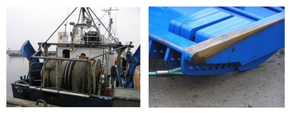
Figure 3. Pelagic trawl doors compared to standard trawl doors in demersal cod trawl fishery.
