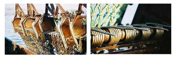
Figure 17. Enviro dredge showing detail of individually sprung teeth (tines).
