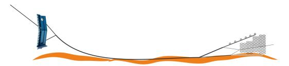
Figure 29. The use of flying/pelagic doors in bottom trawls
