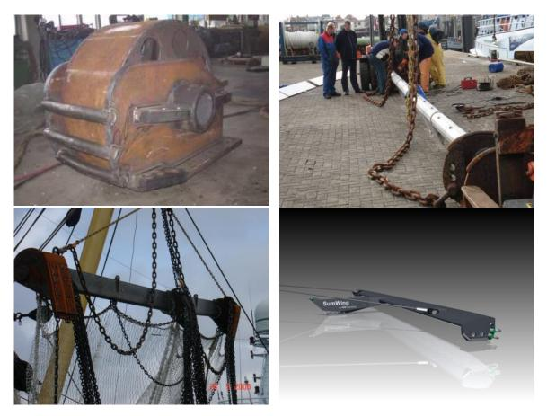
Figure 10. (A) Wheel to replace beam trawl shoe; (B) Spoiler; (C) Fly-beam and (D) SumWing with front runner.
