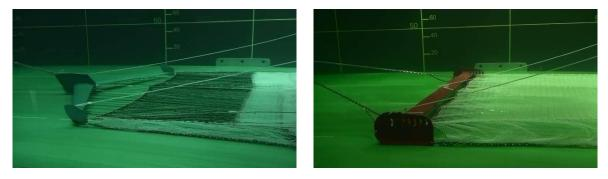
Figure 11. (A) Model of a "Jack Wing" in the flume tank of IFREMER in Boulogne-sur-Mer; (B) Model of a "Delmeco Wing" in the flume tank of IFREMER in Boulogne-sur-Mer.
