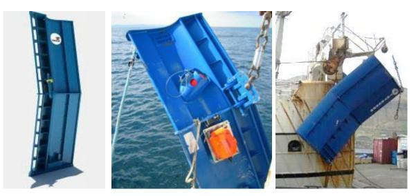
Figure 20. VF15 pelagic otterboard from Thyboron (Denmark).
