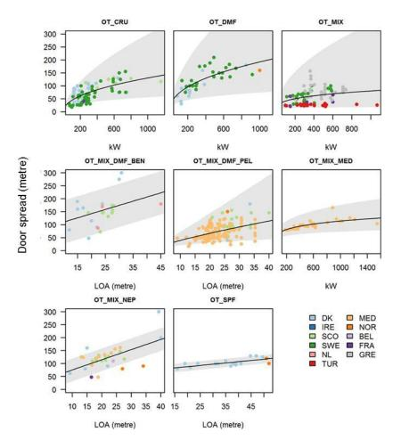
Figure 2. Relationship between total gear width (door spread) and vessel size (kW or overall length) by BENTHIS metier for otter trawlers (OT).
