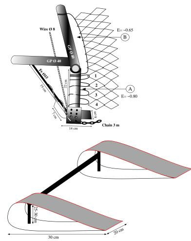
*Figure 1. The technical drawing of the shoes (upper) in traditional beam trawl and the sledges (below) attached to the modified gear (H. Kaykaç, May, 2014)*
