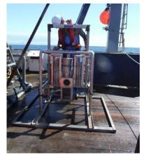
Figure 5. Sediment Profile Imaging (SPI) camera used to measure the apparent redox discontinuity layer as a proxy for bioturbation
