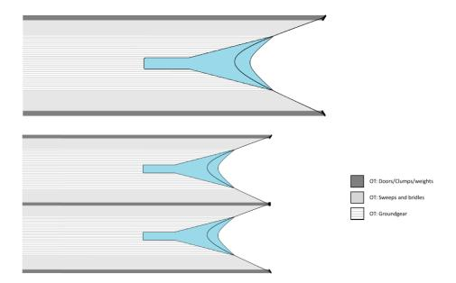
Figure 1: Seafloor footprint of a single otter trawl (top) and a twin-rigged otter trawl (bottom).
