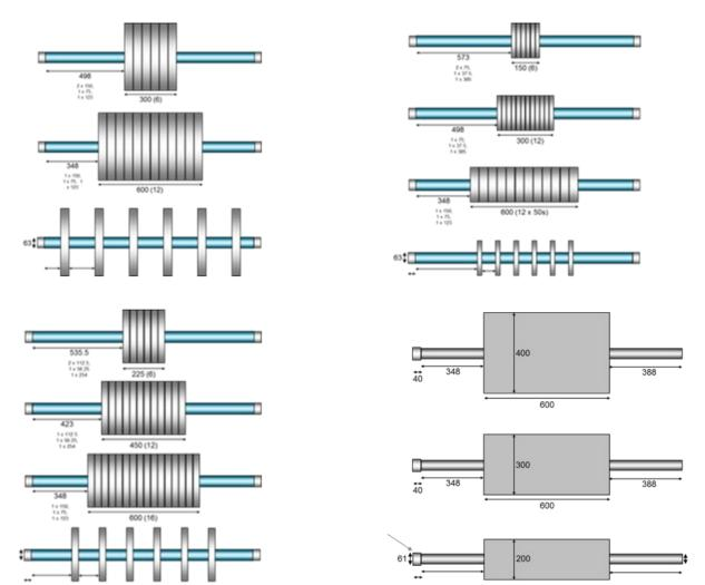
*Figure 2. Illustrations of some of the trawl gear components that are in contact with the seabed that have been tested : cylindrical clumps, disc and rockhopper ground gears, and trawl otter boards.*
