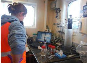
Figure 4. Calibrating the Oxygen probe to measure changes in oxygen concentration with sediment depth
