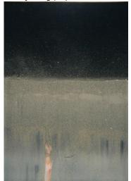
Sediment profile 2 h after beam trawl fishing (T1)
