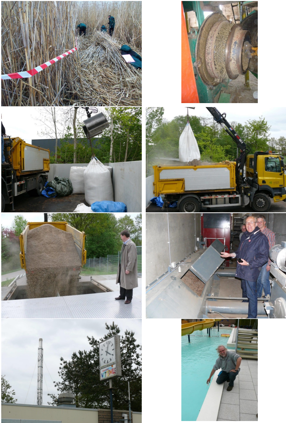
Figure 22 Reed harvested at Gorodische (Ukraine) was pelleted and 10 tons were transported in Big Bags to Marum (The Netherlands) for use in the local wood chip municipal heating plant. At that moment of testing the heat was mainly used for heating the local swimming pool.
